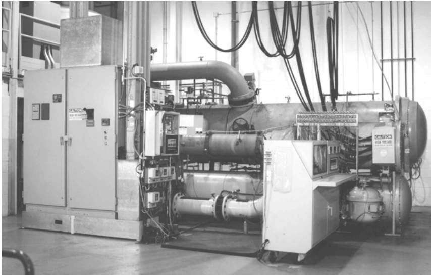
Figure 9 , McQuay's million-dollar compressor test stand with advanced data acquisition provides comprehensive information on new compressor designs.
